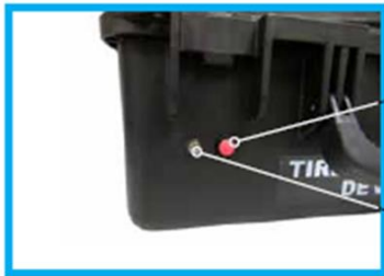
External Check Button Status LED
