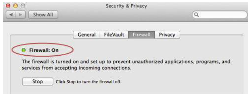
Figure 34: Turning on firewall
