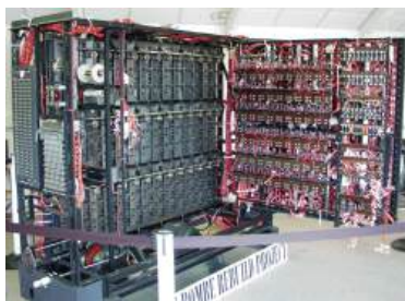
A complete and working replica of the computer Turing invented to break the Enigma cypher, called a “Bombe”, at the British National Museum of Computing at Bletchley Park.
