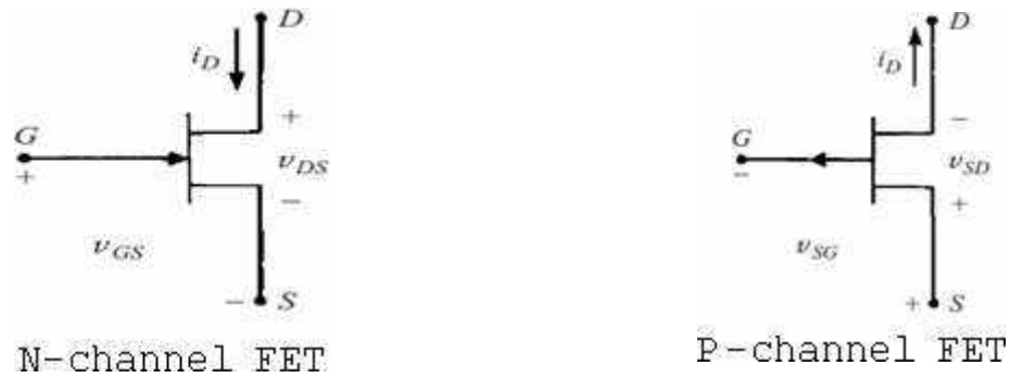
Fig 5.1 schematic symbols for the P-channel and N-channel JFET
