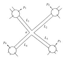
For water at 20°C, take  $\rho$  = 998 kg/m³ and  $\mu$  = 0.001 kg/m.s. All pipes are cast iron, with  $\epsilon/d$  = 0.26/80 = 0.00325. All pipes have L/d = 45/0.08 = 562.5. One solution method is to guess the junction pressure  $p_a$ , iterate to calculate the friction factors and flow rates, and check to see if the net junction flow is zero:
