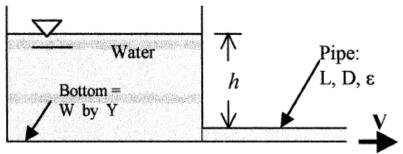
With no driving pressure and negligible tank surface velocity, the energy equation can be combined with a control-volume mass conservation:
