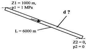
(b) Which is more important to this problem, the head loss due to elevation difference, or the head loss due to pressure dorp in the pipe? (c) Find the minimum required pipe diameter.
