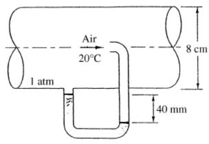
For air at 20°C and 1 atm, take  $\rho$  = 1.2 kg/m³ and  $\mu$  = 1.8E–5 kg/m.s. For water at 20°C, take  $\rho$  = 998 kg/m³ and  $\mu$  = 0.001 kg/m.s. The manometer reads
