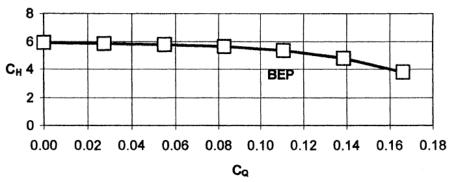
(c) For kerosene,  $\rho_k$  = 804 kg/m³. Convert 7000 gal/min = 0.442 m³/s. At BEP, we require the above values of dimensionless parameters:
