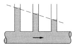
No, this is not an open-channel flow. The open tubes are merely piezometer or pressure-measuring devices, there is no flow in them. The dashed line represents the pressure distribution in the tube, or the "Hydraulic Grade Line" (HGL).
