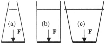
The three free bodies are shown below. Pressure on the side-walls balances the forces. In (a), downward side-pressure components help add to a light W. In (b) side pressures are horizontal. In (c) upward side pressure helps reduce a heavy W.
