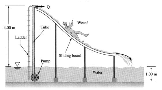
For water take  $\rho$  = 998 kg/m³ and  $\mu$  = 0.001 kg/m·s. Write the steady-flow energy equation from the water surface (1) to the outlet (2) at the top of the slide:
