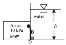
The minimum height needed to open the gate can be assessed by calculating the hydrostatic force on each side of the gate and equating moments about the hinge. The air pressure causes a force,  $F_{air}$ , which acts on the gate at 0.15 m above point D.
