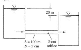
For water at 20°C, take  $\rho$  =998 kg/m³ and  $\mu$  = 0.001 kg/m.s. The energy equation should include the orifice head loss and the entrance and exit losses:
