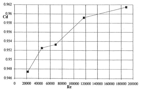
They closely resemble the "classical Herschel venturi," but this data is actually for a modern venturi, for which we only know the value of  $C_d$  for 1.5E5 <  $R_{eD} \le 2E5$ :
