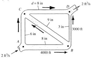
For water at 20°C, take  $\rho$  =1.94 slug/ft³ and  $\mu$  = 2.09E-5 slug/ft.s. Each pipe has a head loss which is known except for the square of the flow rate:
