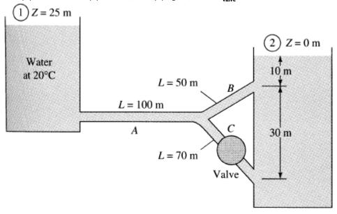
For water at 20°C, take  $\rho$  = 998 kg/m³ and  $\mu$  = 0.001 kg/m.s. For cast iron,  $\epsilon$  ≈0.26 mm, hence  $\epsilon/d$  = 0.26/80 ≈ 0.00325 for all three pipes. Note  $p_1$  =  $p_2$ ,  $V_1$  =  $V_2$  ≈ 0. These are long pipes, but we might wish to account for minor losses anyway:
