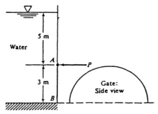
The centroid of a semi-circle is at  $4R/3\pi \approx 1.273$  m off the bottom, as shown in the sketch at right. Thus it is 3.0 - 1.273 = 1.727 m down from the force P. The water force F is
