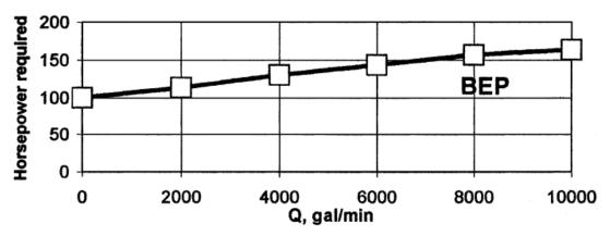
51. A 6.85-in pump, running at 3500 rpm, has the measured performance at right for water at 20°C. (a) Estimate the horsepower at BEP. If this pump is rescaled in water to provide 20 bhp at 3000 rpm, determine the appropriate (b) impeller diameter; (c) flow rate; and (d) efficiency for this new condition.
