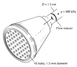
For water at 50°C, take  $\rho$  =988 kg/m³ and  $\mu$  = 0.548E-3 kg/m.s. Further assume that the shower head is a poor diffuser, so the pressure in the head is also about 400 kPa. Assume the outside pressure is sea-level standard, 101 kPa. Estimate  $C_d \approx 0.61$ . Then, with  $\beta \approx 0$  for the small holes, each hole delivers a flow rate of
