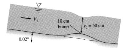
For brickwork, take  $n \approx 0.015$ . Since the water level decreases over the bump, the upstream flow is subcritical. For a wide channel,  $R_h = y/2$ , and
