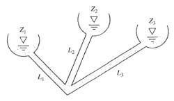
For water at 20°C, take  $\rho$  = 998 kg/m³ and  $\mu$  = 0.001 kg/m.s. All pipes have  $\epsilon/d$  = 1/280 = 0.00357. Let the intersection be "a." The head loss at "a" is desired:
