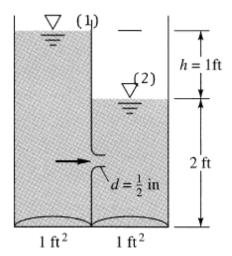
For water at 20°C, take  $\rho$  =1.94 slug/ft³ and  $\mu$  = 2.09E-5 slug/ft.s. For a long-radius nozzle with  $\beta \approx 0$ , guess  $C_d \approx 0.98$  and  $K_{loss} \approx 0.9$ . The elevation difference h must balance the head losses in the nozzle and submerged exit:
