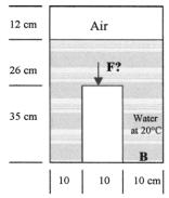
(a) The pressure in the air space can be found by working upwards hydrostatically from point  $\mathbf{R}$ .
