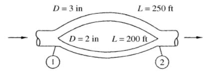
For SAE 10 oil at 20°C, take  $\rho$  = 1.69 slug/ft³ and  $\mu$  = 0.00217 slug/ft.s. For cast iron,  $\epsilon \approx 0.00085$  ft. Convert  $\Delta p$  = 3 psi = 432 psf and guess laminar flow in each:
