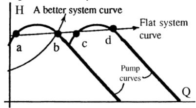
As discussed, for one pump with a flat system curve, point a is statically unstable, point b is stable. A 'better' system curve only passes through b. For two pumps in parallel, both points a and c are unstable (see above). Points b and d are stable but for large disturbances the system can 'hunt' between the two points.
