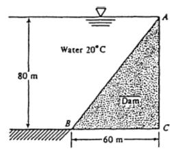
The centroid of surface AB is 40 m deep, and the total force on AB is
