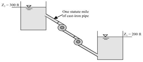
For water at 20°C, take  $\rho$  = 1.94 slug/ft³ and  $\mu$  = 2.09E-5 slug/ft·s. For cast iron,  $\epsilon \approx 0.00085$  ft. The 35-inch pump has the BEP values  $Q^* \approx 18$  kgal/min,  $H^* \approx 190$  ft. In series, each pump takes H/2, so a BEP series operation would match
