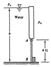
The centroid of AB is 2.0 ft below A, hence the centroidal depth is h + 2 - 4 = 7.5 ft. Then the total hydrostatic force on the gate is
