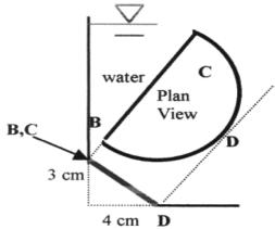
(a) The radius of BCD is 5 cm. Its centroid is at  $4R/3\pi$  or  $4(5 \text{ cm})/3\pi = 2.12 \text{ cm}$  down along the slant from BC to D. Then the vertical distance down to the centroid is  $h_{CG} = 8 \text{ cm} + (2.12 \text{ cm}) \cos (53.13^\circ) = 9.27 \text{ cm}$ .
