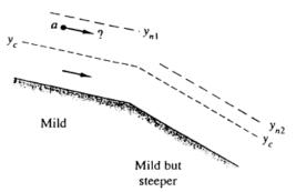
There are two possible profiles, depending upon whether or not the initial M-2 profile slips below the new normal depth  $y_{n2}$ . These are shown on the next page:
