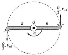
Utilizing the velocity diagram at right, we apply the Euler turbine formula:
