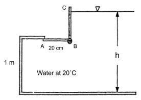
Let H = (h - 1 meter) be the depth down to the level AB. The forces on AB and BC are shown in the free body at right. The moments of these forces about B are equal when the gate opens:
