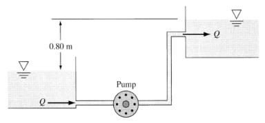
For water, take  $\rho = 998 \text{ kg/m}^3$  and  $\mu = 0.001 \text{ kg/m} \cdot \text{s}$ . NOTE: The tubing is so small that the flow is laminar, even at the highest pump flow rate:
