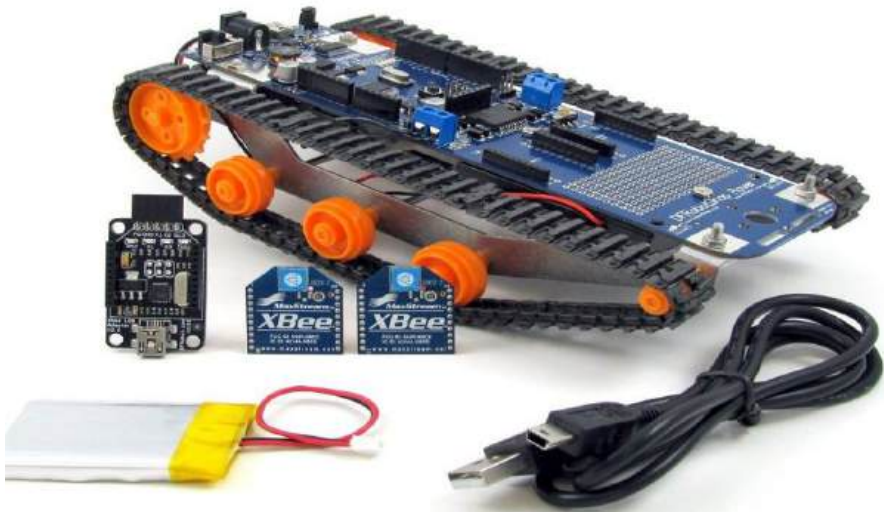
Figure 1.10 Tank Robot DFRobot Rover ver.2 using Arduino and XBee for Wireless Communication (source:robotshop.com).
