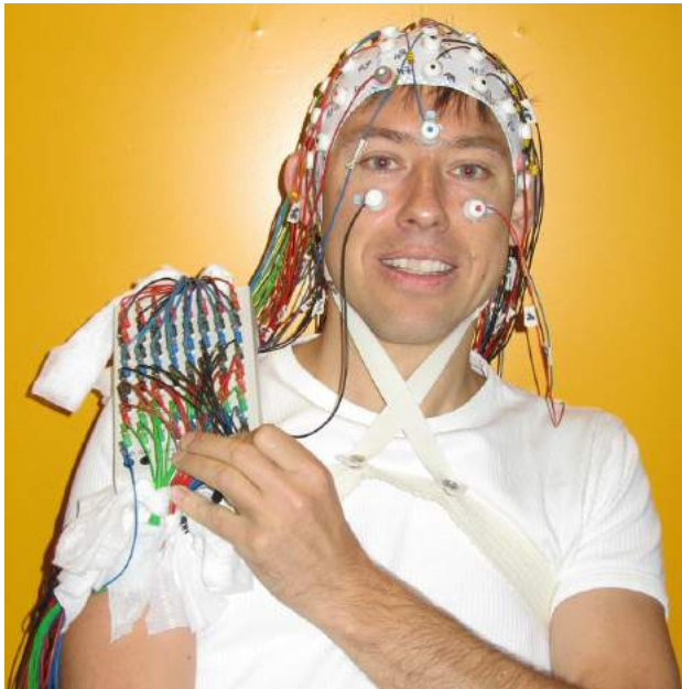
Figure 2: This man is wearing an elastic electrode cap into which individual electrodes (inside the white circles) are sewn into standardized locations. [Image: Hans, CC0 Public Domain, https://goo.gl/m25gce ]
