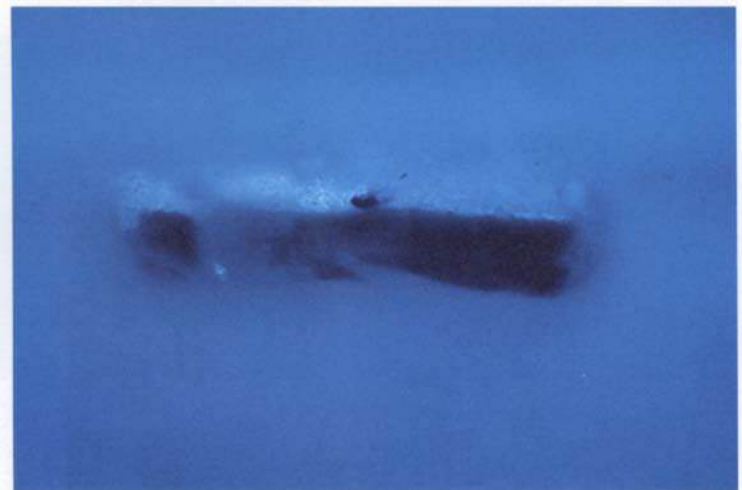
Plate 12. Cross section from Palmezzano's Mystic Marriage of Saint Catherine, showing the oiling-out layer between the underpainting and the final glaze in UV light (×220). Photograph by Christopher Hurst. Private collection.
