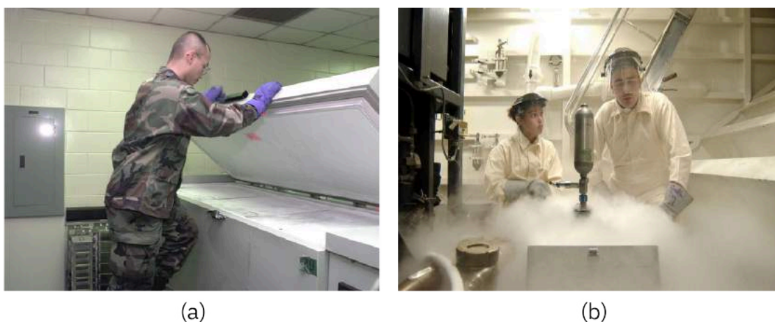
Figure 13.10 Cultures and other medical specimens can be stored for long periods at ultra-low temperatures. (a) An ultra-low freezer maintains temperatures at or below -70^{\circ}\text{C} . (b) Two people stand in a room with a large nitrogen storage unit emitting a large amount of fog. (credit a: modification of work by “Expert Infantry”/Flickr; credit b: Credit: US Navy; Public Domain.)
