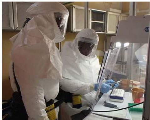
Figure 6.15 Researchers working with Ebola virus use layers of defenses against accidental infection, including protective clothing, breathing systems, and negative air-pressure cabinets for bench work. (credit: modification of work by Randal J. Schoepp)
