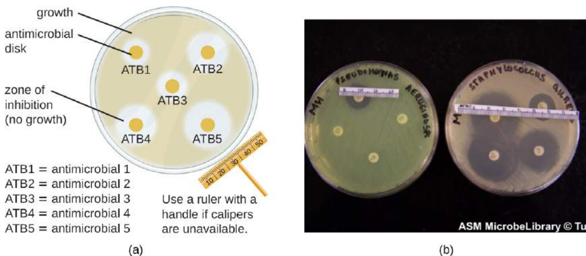
Figure 13.31 A disk-diffusion assay is used to determine the effectiveness of chemical agents against a particular microbe. (a) A plate is inoculated with various antimicrobial discs. The zone of inhibition around each disc indicates how effective that antimicrobial is against the particular species being tested. (b) On these plates, four antimicrobial agents are tested for efficacy in killing Pseudomonas aeruginosa (left) and Staphylococcus aureus (right). These antimicrobials are much more effective at killing S. aureus , as indicated by the size of the zones of inhibition. (credit b: modification of work by American Society for Microbiology)
