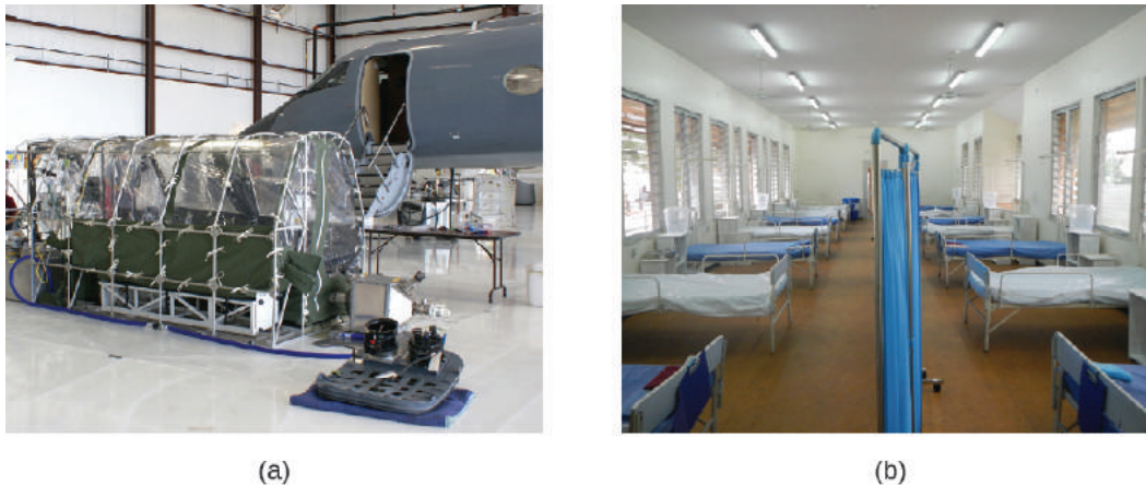
Figure 16.15 (a) The Aeromedical Biological Containment System (ABCS) is a module designed by the CDC and Department of Defense specifically for transporting highly contagious patients by air. (b) An isolation ward for Ebola patients in Lagos, Nigeria. (credit a: modification of work by Centers for Disease Control and Prevention; credit b: modification of work by CDC Global)
