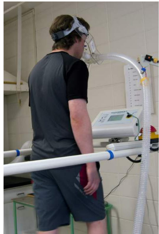
Figure 2.2: Student performing a graded exercise test on a treadmill. A headpiece connects to a mouthpiece with a set of one-way valves which allows for transfer of expired gases via a collection tube to a metabolic cart for analysis of carbon dioxide and oxygen concentrations. A nose clip ensures that expired air is only leaving through the mouth.
