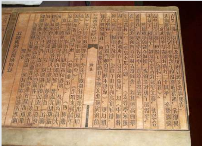
Figure 4.23 | A woodblock used to print one page of classical Chinese | The characters read from top to bottom and right to left. During the Song, individual, moveable woodblocks with one character were also carved and arranged in square frames.
