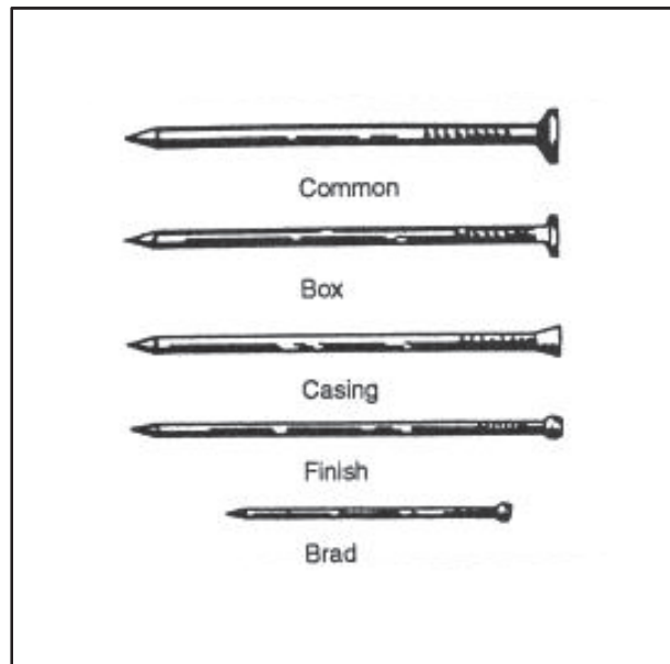
Figure 2-4. Types of nails
