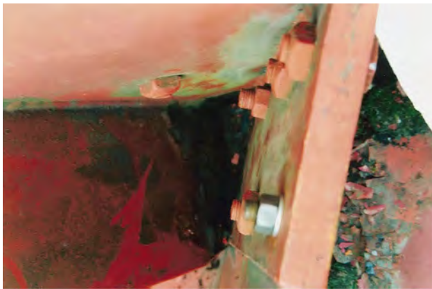
Figure 9 In the corners of the sculpture, pockets form where water can collect, leading to corrosion. © 2014 Calder Foundation, New York / Artists Rights Society (ARS), New York. © ZMK, Hannover 2003.
