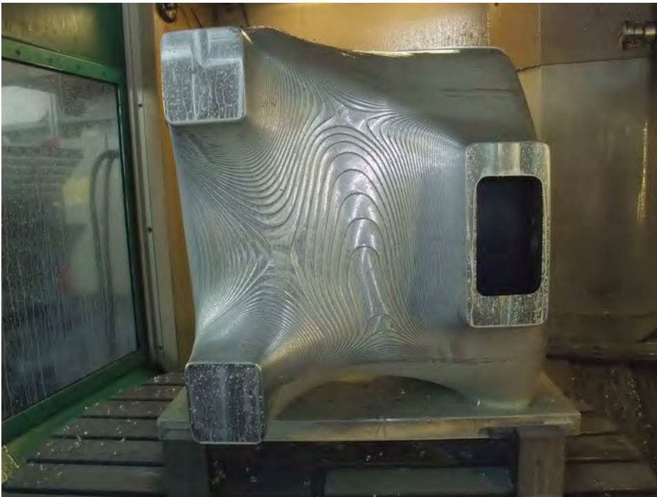
Figure 3 A form block from Philosophy undergoing the first step, rough filing, during the 5-axial milling process. Used with permission of Anselm Reyle. Photo: Thomas Dempwolf.
