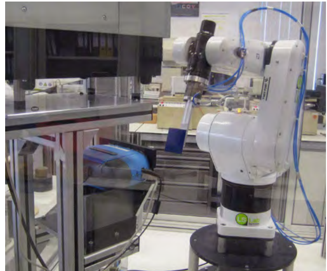
Figure 4 An automated robot was used to take color and gloss measurements during and after aging tests at AkzoNobel. Photo by Nikki van Basten.
