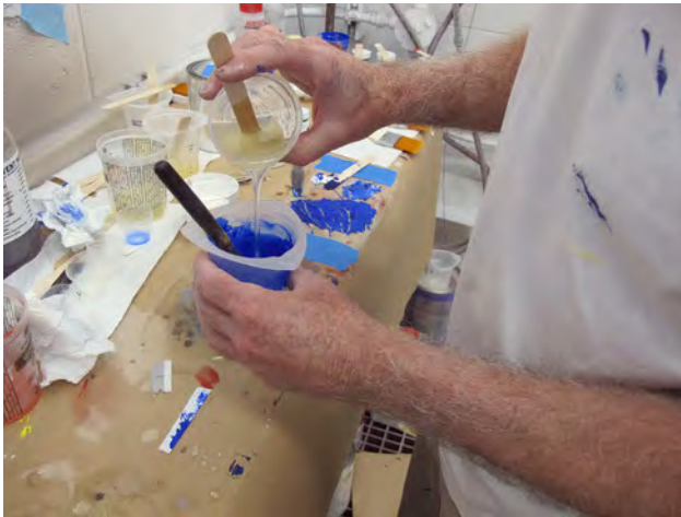
Figure 9 The MSA is mixed with the IIS clear coat to make the top glaze for the blue color field. © Estate of Roy Lichtenstein. Photo by Julie Wolfe.
