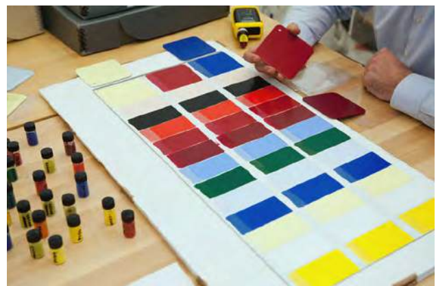
Figure 10 Comparison of trial paint swatches from Roy Lichtenstein’s studio and a fabricator. The creation of sets of such paint coupons, made to an agreed-upon size and format, was identified during the symposium as a priority of the field.
