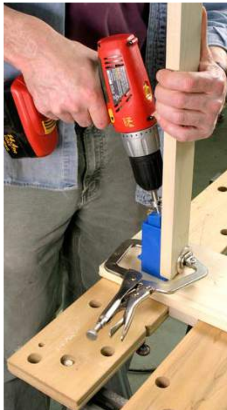
Use the high speed setting on your drill to make the pocket hole.
