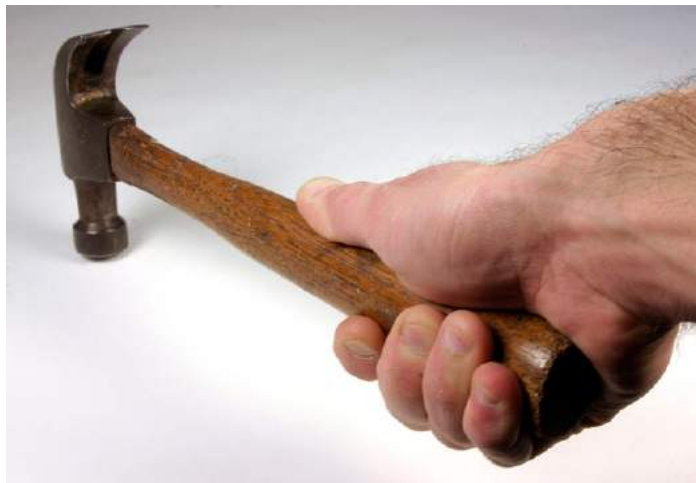
This is the power stroke with a hammer. When you build a deck, or really anything, grip the tool at the end of the handle. Sticking your thumb out will help steady the tool a bit.
