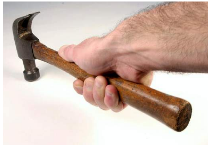
By choking up on the handle you can gain some finesse and reduce the force you transmit into the nail (sometimes a good thing, really). Note again the position of my thumb.
