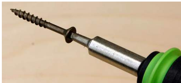
The square drive holds so well that the screw will hang on the end of the bit.
