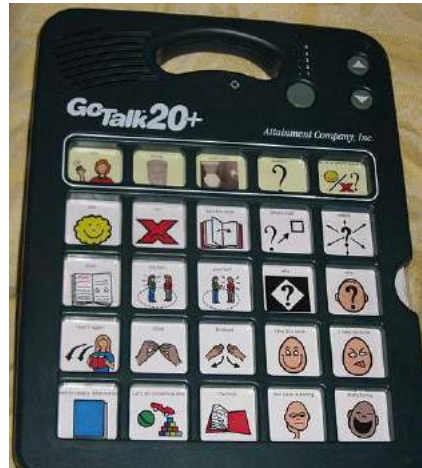
Figure 9.18 Go Talk Static communication device 318
