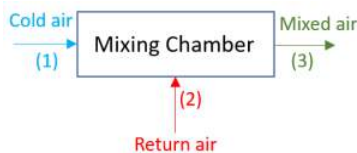
Figure 5.3.10 Schematic of a mixing chamber in HVAC (heating, ventilating and air conditioning) system
