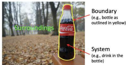
Figure 1.2.2 A sealed bottle of soft drink as an example of closed systems
