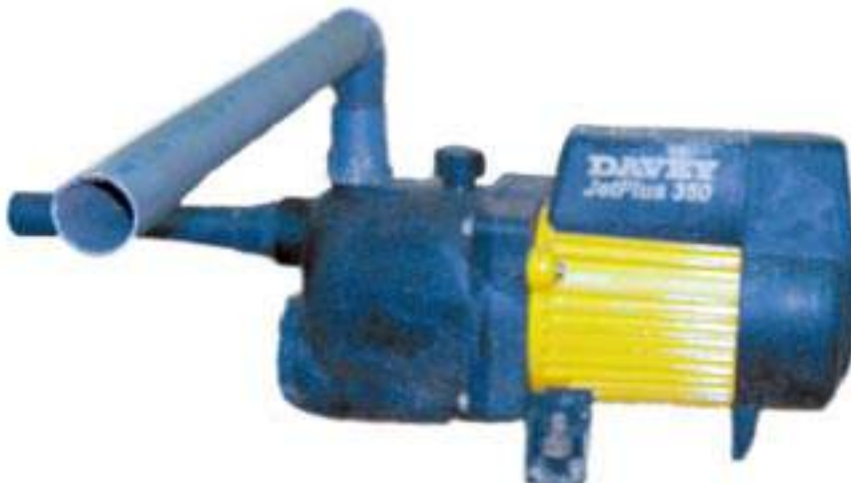
Figure 65: A domestic water pump
