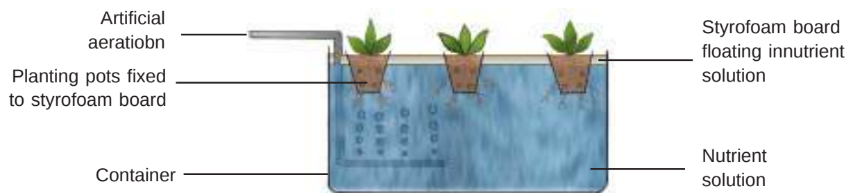
Figure 21: Diagrammatic view of floating technique
