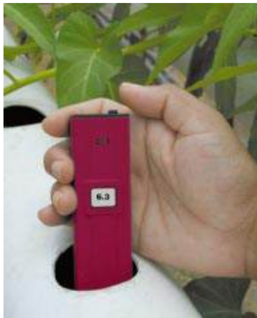
Figure 39: Measuring nutrient solution pH using a portable digital pH meter
