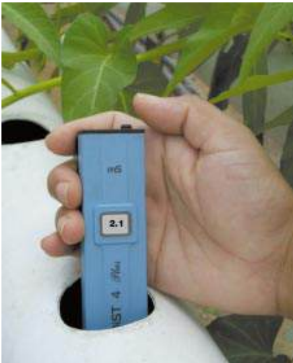
Figure 41: Measuring nutrient solution Ec using a portable digital Ec meter
