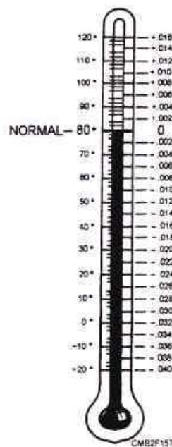
Figure 2-4.- Hydrometer conversion chart.
