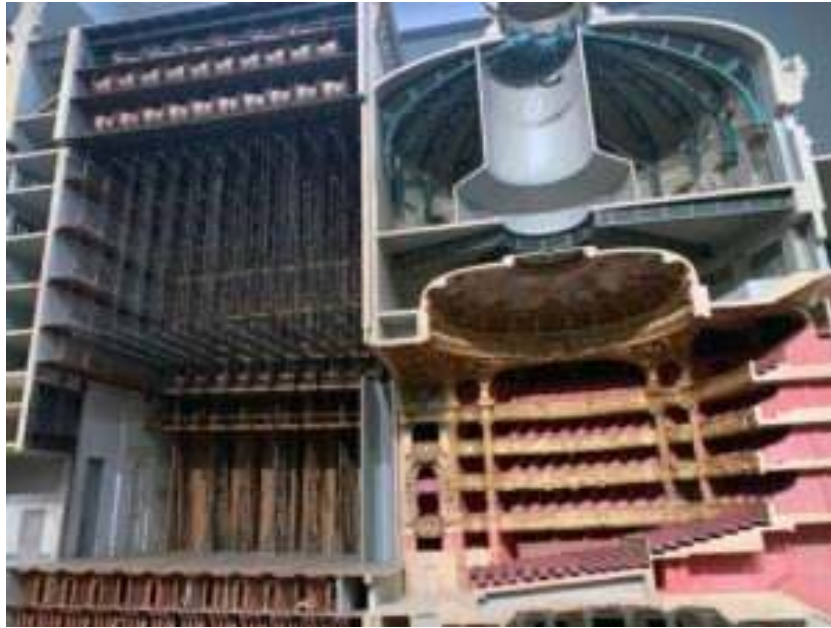
Model of the Garnier Opera House, Paris. You can see the fly loft over the stage on the left, and the house with the stalls on the right. Photo by Kiara Pipino
