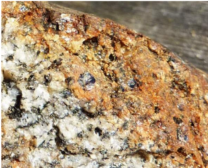
Figure 5.1.4: A granitic rock containing biotite and amphibole which have been altered near to the rock's surface to limonite, which is a mixture of iron oxide minerals.
