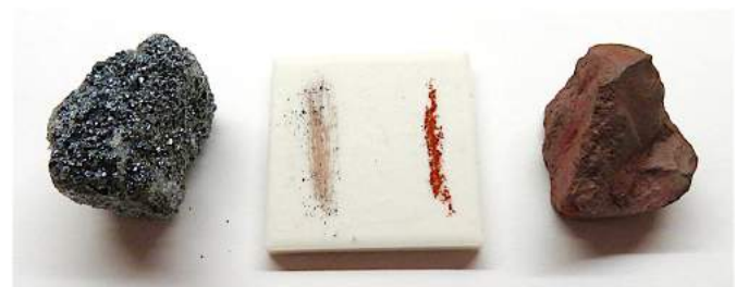
Figure 2.3.2 The streak colours of specular (metallic) hematite (left) and earthy hematite (right). Hematite leaves a distinctive reddish-brown streak whether the sample is metallic or earthy.
