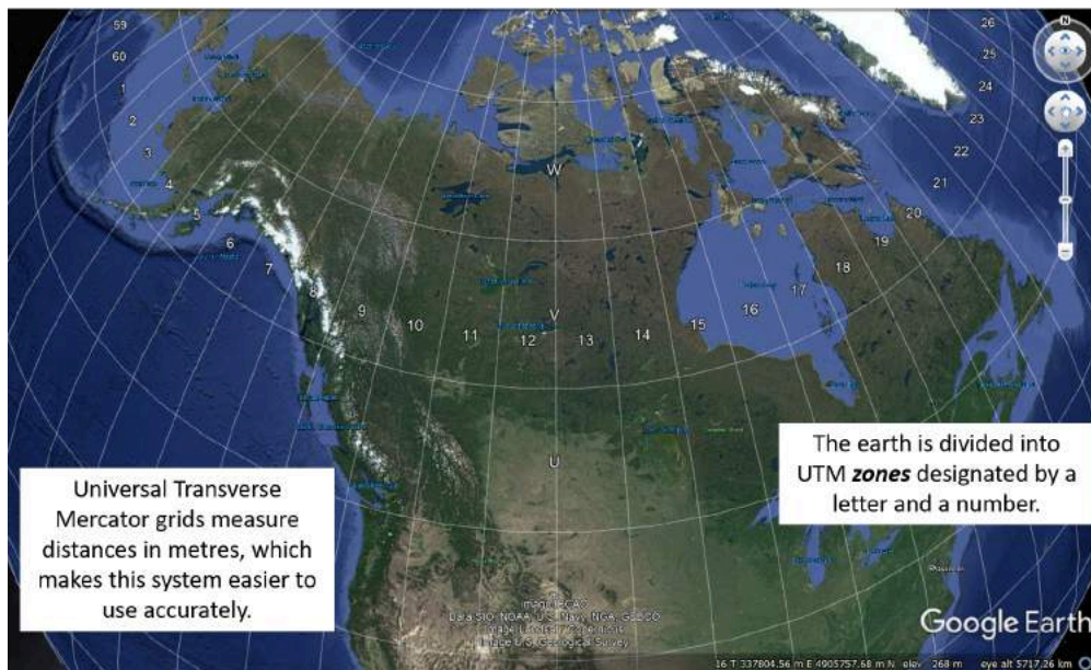
Figure T10: Universal Transverse Mercator (UTM) zones in Canada. Zones are designated by a number and a letter, e.g., the city of Vancouver, BC is in UTM zone 10 U.
