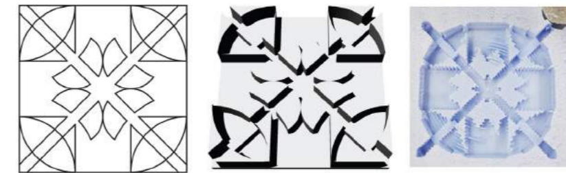
Figure 4: Three stages of the model generation (from left): Generating a 2d pattern, 3d modeling of a surface based on the pattern, CNC-milled material outcome (Image courtesy: Nazlı Babar Ursavaş)
