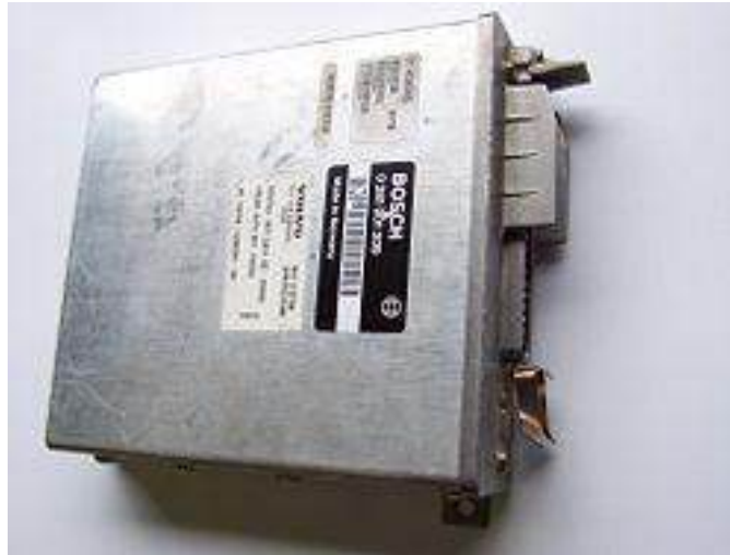
EDC control unit
