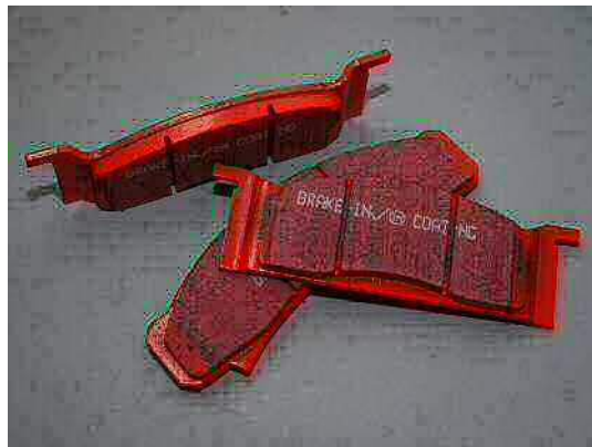
Disc brake pads. They're red in this image. They can be any color.
