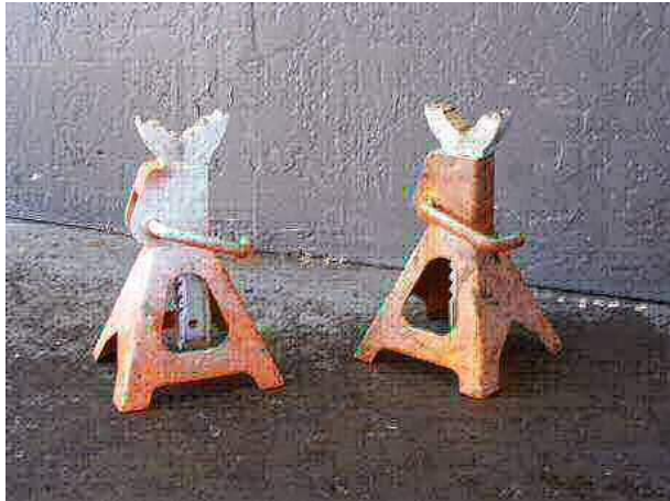
Two jack stands, the lever shown on these stands is not used to raise the vehicle but to adjust the height of the stands to keep the vehicle raised.
