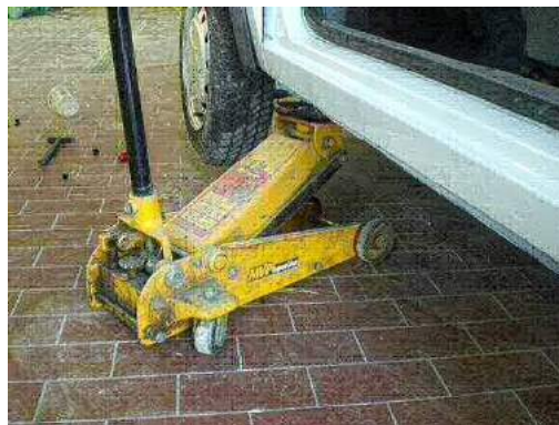
Hydraulic jack with hand-pump mechanism
