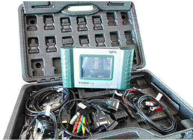
Auto scanner which receives DTCs from the vehicle's computer Image credit: CC-BY-SA-Florian Schaffer
