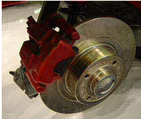
A disc brake. The rotor is the shiny gold-colored disc and the caliper is red. The black piece between the caliper and the rotor is the pad.
