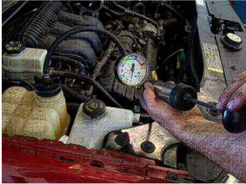
Pressure testing the cooling system
