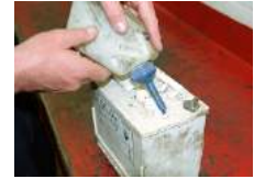
Open cell battery - with removable caps
