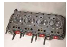
Core plugs and coolant holes
