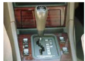
A switch makes when in the park and neutral position
