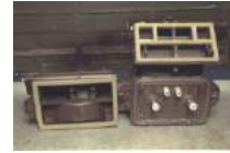
Heater air control flaps
