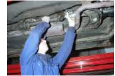
Checking the universal joints
