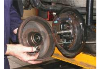
Leading and trailing system
