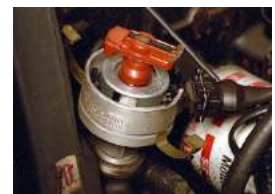
Distributor for engine speed and position sensing
