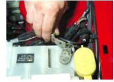
Removing the earth lead
