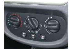
Air conditioning controls
