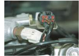
Air temperature sensor
