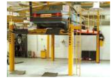
Four post lift in use
