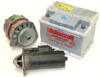
Battery, starting and charging components
