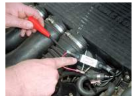
50A ammeter shunt
