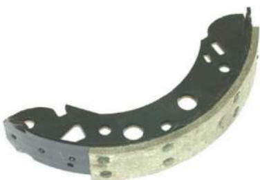
Brake lining riveted to a shoe
