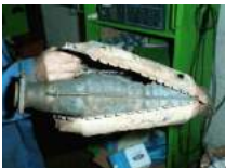
A damaged catalytic converter
