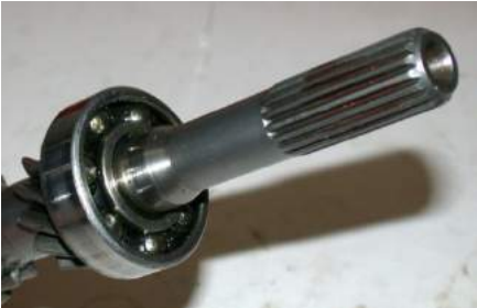
This bearing on a gearbox shaft is held in place by compression
