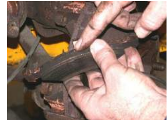
Checking the pad lining thickness
