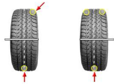
Wheels that have been statically balanced
