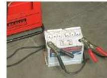
Battery caps removed during fast charging
