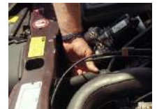
Engine is up to temperature when the top hose is hot
