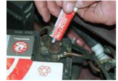
Clean and apply battery grease
