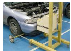
Beam setter in use
