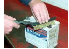
Cleaning the battery terminals
