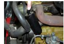
Oil separator connected to the crankcase
