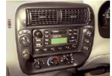
Fresh air fascia vents
