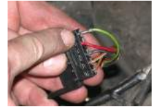
Damaged wiper motor connections
