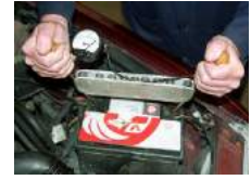
A good battery under test
