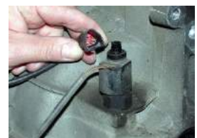
Road speed sensor in position
