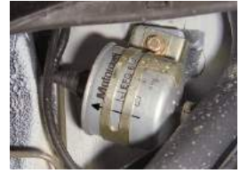
Filters are directional
