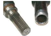
A splined joint connects to the gearbox
