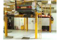
Four post lift in use
