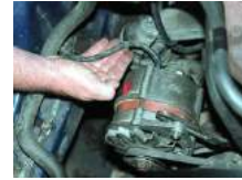
Alternator cables to battery
