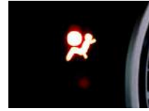
SRS warning light
