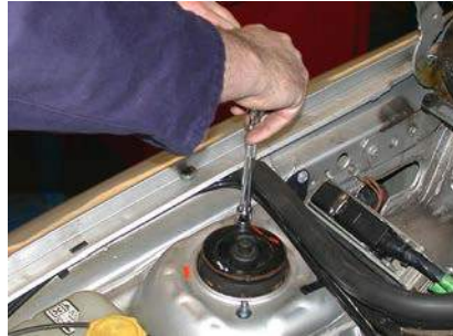
This damper is part of the strut
