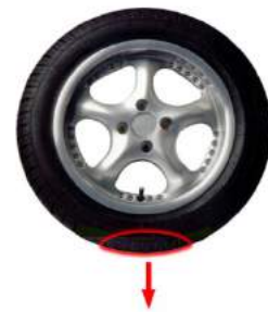
Wheel with an out of balance mass
