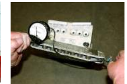
Battery heavy duty discharge test
