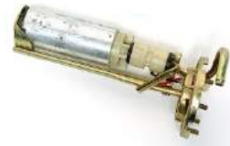
Electric fuel pump in the tank
