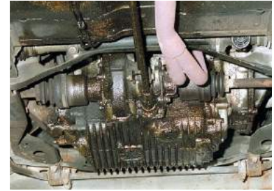
This oil leak was obvious!
