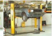
Two post lift in use
