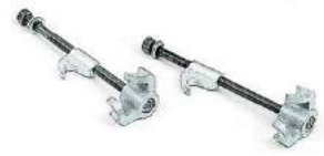
McPherson strut springs must be compressed for removal
