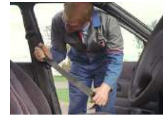
Checking the belt condition
