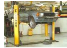
Two post lift in use
