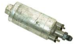
Electric fuel pump in the line
