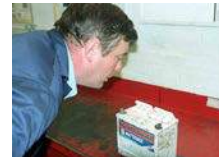
Blow away any hydrogen gas before starting the test
