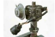
Distributor with vacuum control
