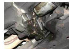
Transmission oil leak
