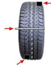
Statically balanced but dynamically imbalanced
