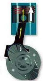
Force transfer from crankshaft to piston crown through the connecting rod
