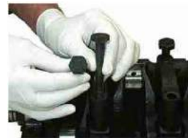
Main bearing bolts
