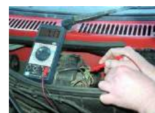
Checking voltage at the resistor pack
