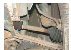
Driveshaft and CV gaiters in position
