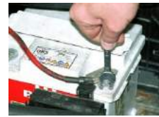
Undoing the battery terminal
