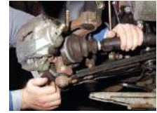
This shaft transmits drive to the wheels
