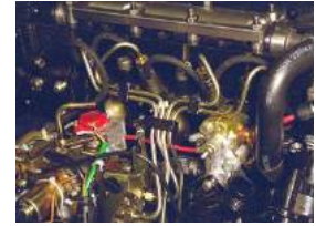
Injection pump, pipes and injectors
