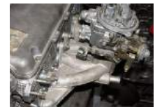
Old inlet manifold
