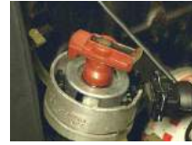
Rotor in place
