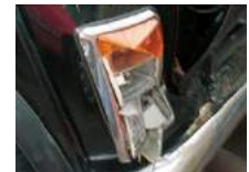
Damaged rear light lens
