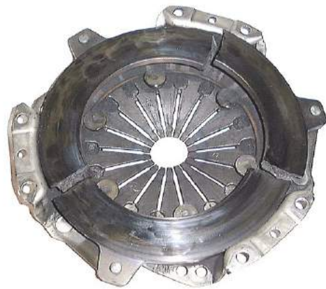
Seriously damaged clutch!
