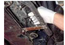
Coolant being drained
