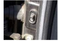
Switch positioned in the door pillar
