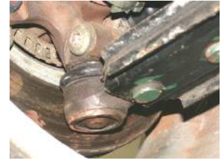
Greasing swivel joints is only necessary on older cars
