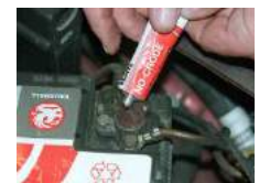
Terminals with battery grease
