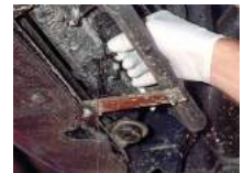
Radiator being drained
