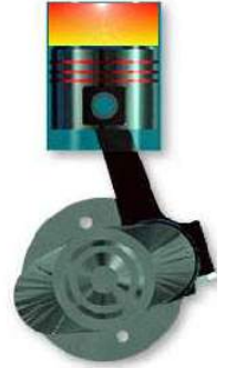
Ideal position for maximum combustion pressure
