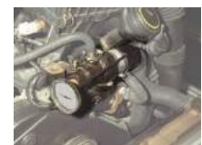
Temperature gauge fitted to test the cooling system
