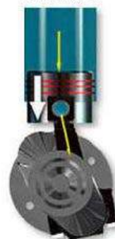
Force transfer from piston crown to crankshaft through the connecting rod
