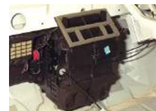
Heater box and flaps
