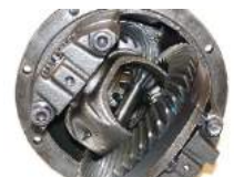
The differential can be called a torque equaliser
