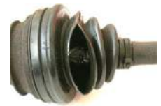
Damaged CV gaiter
