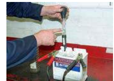
Checking batteries on charge with a hydrometer
