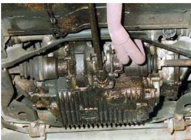
This oil leak was obvious!
