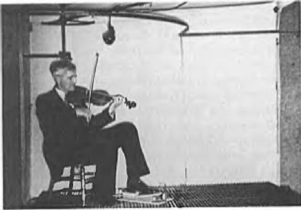
FIG. 9. Professor F. A. Saunders testing a violin in the especially built corner of the Cruft Acoustical Laboratory, Harvard University. (Courtesy of F. A. Saunders.)
