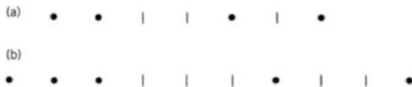
Fig. 5.10 Two linear array configurations in which the antennas are represented by filled circles. (a) Arsac's (1955) configuration containing all spacings up to six times the unit spacing, with no redundancy. (b) Bracewell's (1966) configuration containing all spacings up to nine times the unit spacing, with the unit spacing occurring twice.
