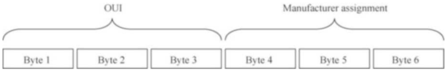
Fig. 7.5 BIA address format
