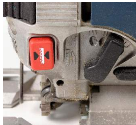
Shown is a properly set jigsaw with the orbital on “1.” When you work in thicker material (or need to saw really fast), switch up to “2” or “3.”
