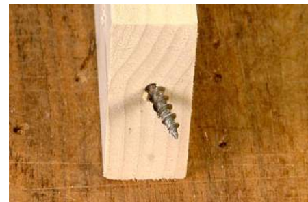
The screw should exit the end of the wood near the center of the board's thickness. Don't worry about getting it precisely placed. The next step will let you know if your setup will work.
