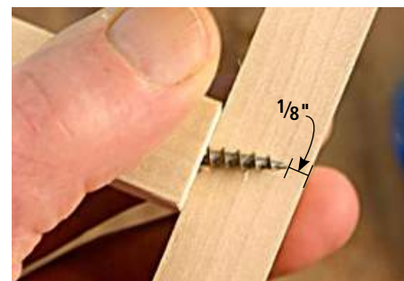
Hold a piece of scrap against the piece with the screw in it. Check to see that the end of the screw is about \frac{1}{8} " away from the surface.
