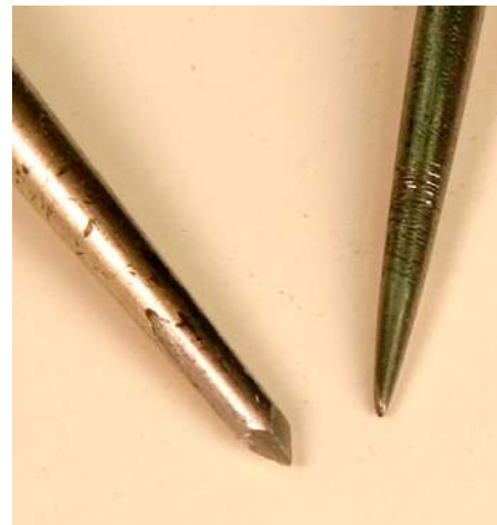
The faceted point on the left makes the awl an efficient tool for making a small hole.
