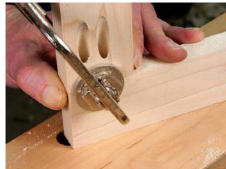
Line up the two pieces and set the clamp to hold them together.
