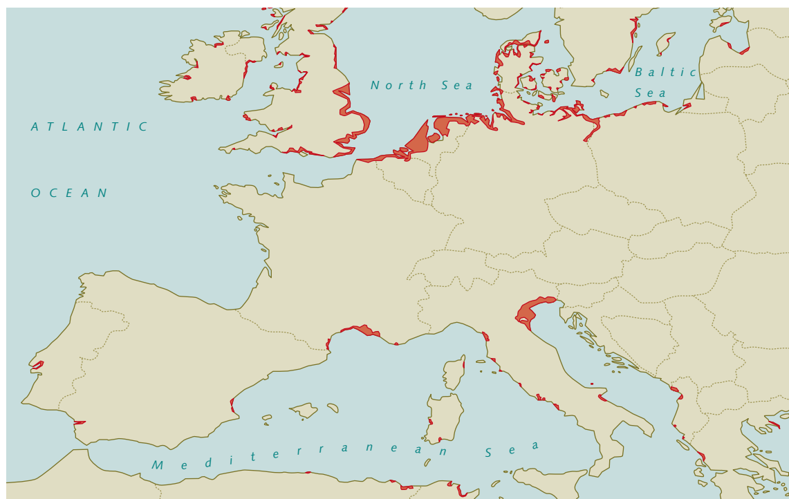
3.10 > If the coasts were not protected by dikes, sea-level rise of 2 metres would produce this picture. The red-coloured areas would be permanently inundated. According to current predictions sea level could rise by as much as 180 cm by the end of this century.
