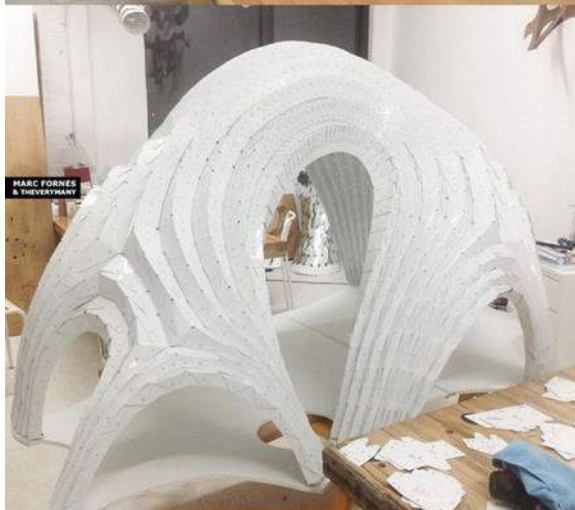
133. Pleated Shell. 1/15 scale structural model Fuente: www.theverymany.com
