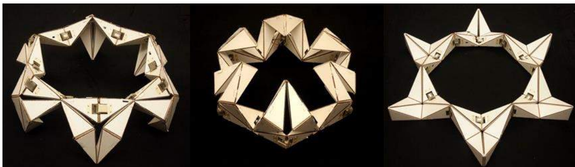
101. HexaMorph: A Reconfigurable and Foldable Hexapod Robot Inspired by Origami.
