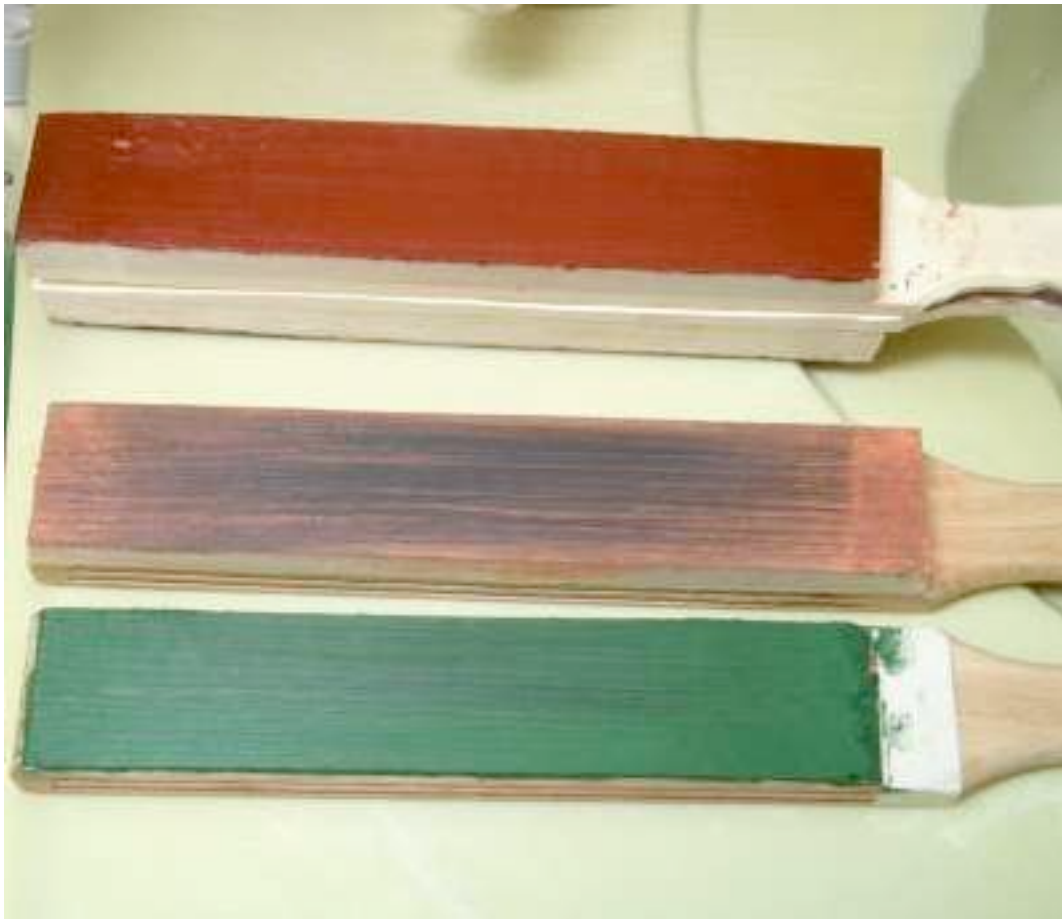
Paddle strops (balsa on wood) with hematite, diamond and chrome oxide pastes.
