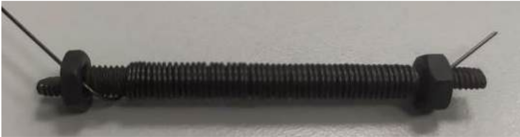
Figure 3.14 Nitinol wire constrain in a screw with two nuts.
