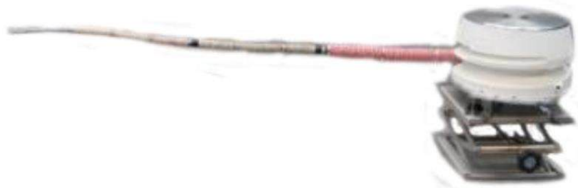
Figure 5.3 Robot with 25 DoF for inspection and reparation tasks in wind turbines [352]
