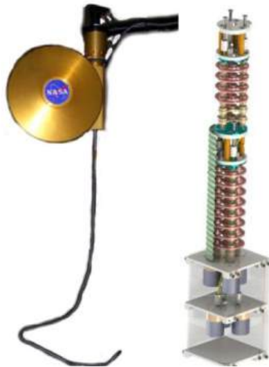
Figure 5.2 (a) Tendril , made by NASA to perform minimally invasive tasks in space [349]. (b) ET ARM , actuated by artificial muscles [350].
