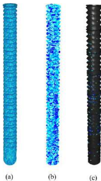
Figure 5.16 (a) Full-order deformation mesh with 120000 tetrahedra, infeasible for real-time applications. (b) The heuristic method adapts a model with 1650 elements to match the real robot behavior. (c) The Model Order Reduction decreases the number of state variables of the model to 1886 while retaining its original characteristics
