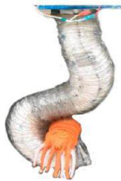
Figure 5.4 Air-Octor, a continuous manipulator robot with multiple sections [30]
