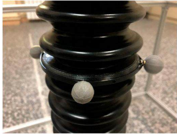
Figure 5.22 Three of a total of twelve infrared-sensitive passive markers used by the motion capture system to obtain the robot pose.
