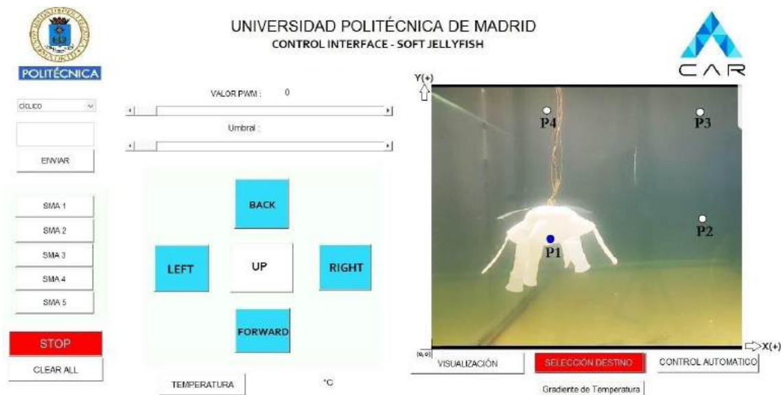
Figure 4.29 Interface for control and configuration in MATLAB
