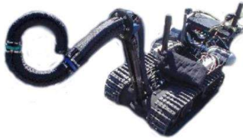
Figure 5.5 Octarm V, a soft robot inspired in an octopus tentacle [4].
