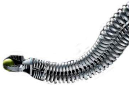
Figure 5.6 Bionic Handling Assistant (BHA) is a pneumatic soft robot with high dexterity made by Festo [31].
