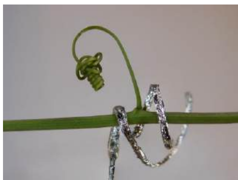
Figure 4.37 Tendril-like soft robot able to climb [340]
