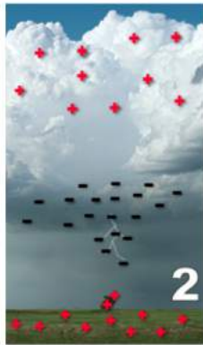
2 Negatively charged area in the storm will send out a charge.
