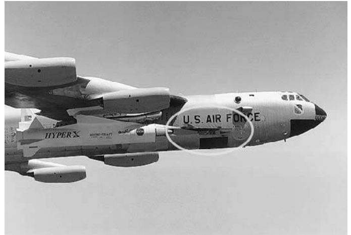
Pegasus with X-43A (in circle) mounted under wing of B-52 launch plane.
