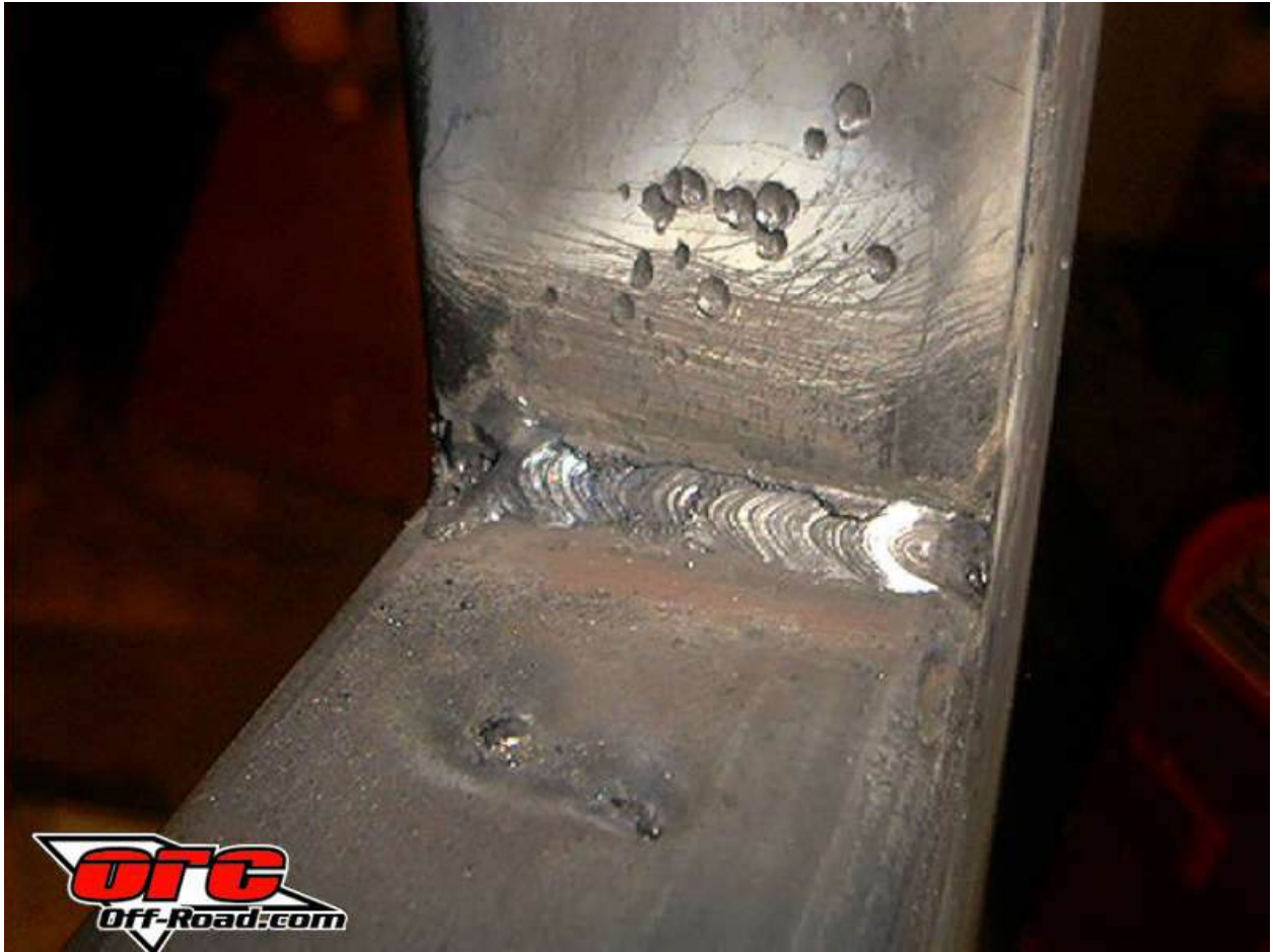
Photo 2: Stick Welding Mild Steel Square Tubing
