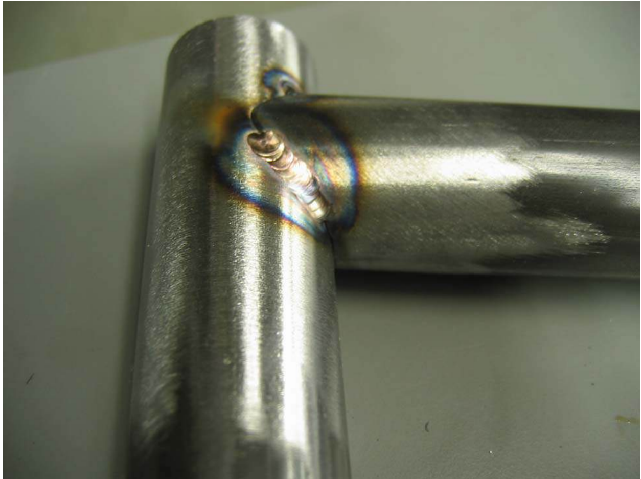
Photo 5: Fillet TIG Weld (4130 Structural Steel Tubing)
