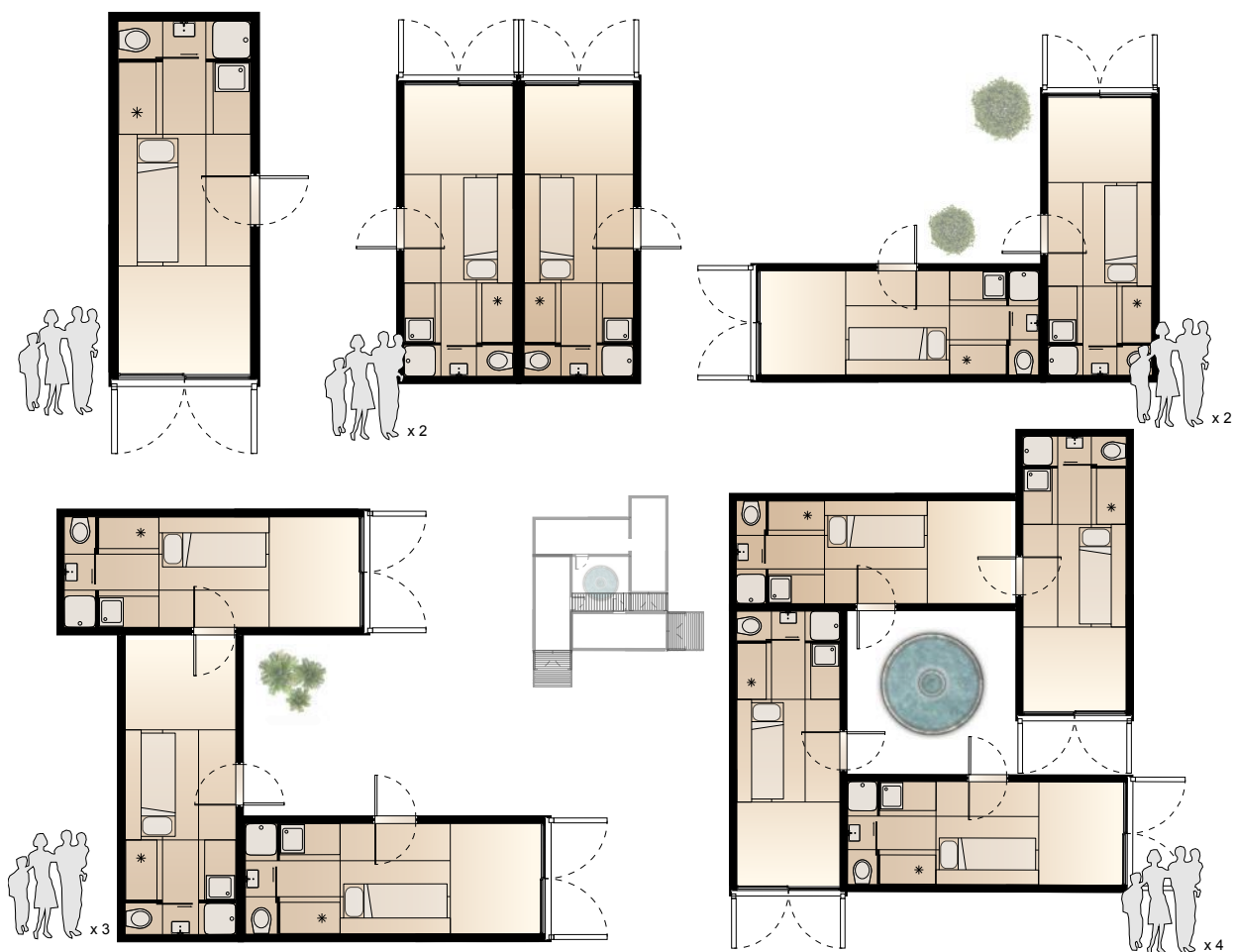
Figure 5.1- The same container and its openings can be put together in countless number of ways and combinations. It is due to its modularity – orthogonal box- that reminds of a gigantic LEGO piece to be played with. (Source: Mafalda Melo Oliveira, 2014)
