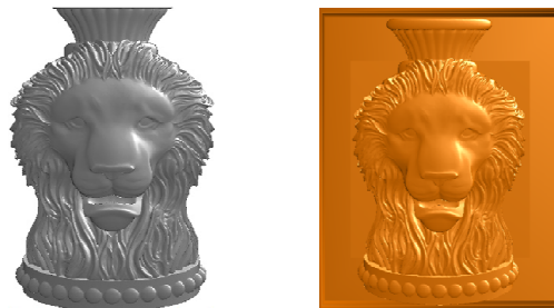
Figure 4. 6 The bas relief generated by the proposed algorithm: Vase lion and rendered Vase lion with frame.
