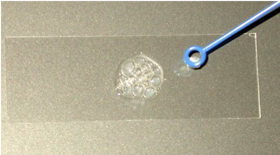
Figure 1. A positive catalase test, as evidenced by the release of “bubbles” of \text{O}_2 .
