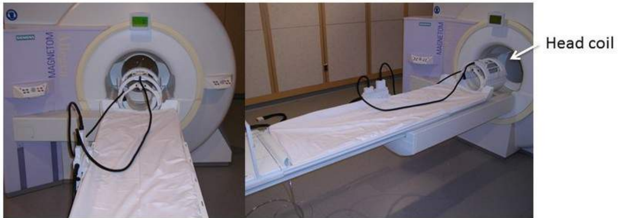
Figure 3. Functional magnetic resonance imaging (fMRI) scanner used to image the brain while people perform tasks. The scanner allows researchers to view the changes in blood oxygenation in specific locations in the brain during a task. Images are collected using powerful magnets and radio waves that shift the position of atoms in oxygenated blood that rushes to areas involved in performing the task. MRIs are non-invasive and there are no known risks from exposure to the magnetic fields or radio waves. Subjects lay on the white bed with their head inside the head coil, then the bed is moved into the scanner.
