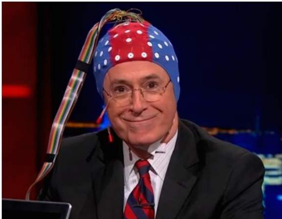
Figure 2: TV host Stephen Colbert demonstrates EEG data collection on the 4/4/13 episode of the Colbert Report. Colbert is wearing an elastic electrode cap into which individual electrodes (inside the white circles) are sewn into standardized locations.
