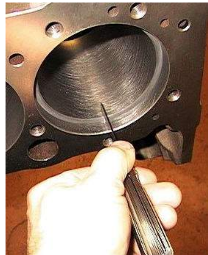
Measuring Piston Ring End Gap
