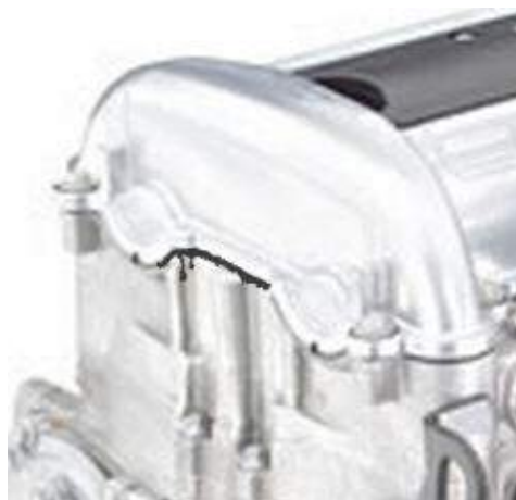
Using Foot Powder for Visual Leak Detection
