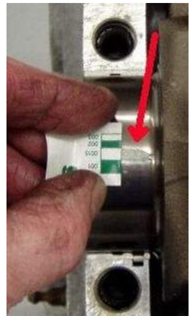
Bearing Clearance Measurement
