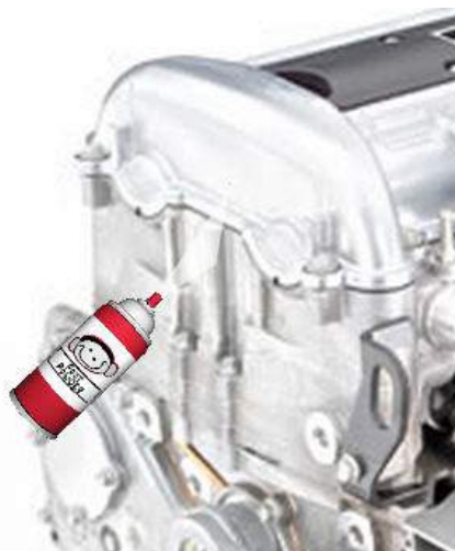
Using Foot Powder for Visual Leak Detection
