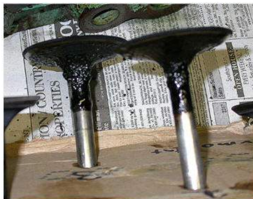
Carbon Deposits on Intake Valve
