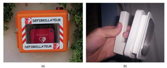
Figure 6.2.10. Defibrillators. (a) An external automatic defibrillator can be used by nonmedical personnel to re-establish a normal sinus rhythm in a person with fibrillation. (b) Defibrillator paddles are more commonly used in hospital settings. (credit b: "widerider107"/flickr.com).
