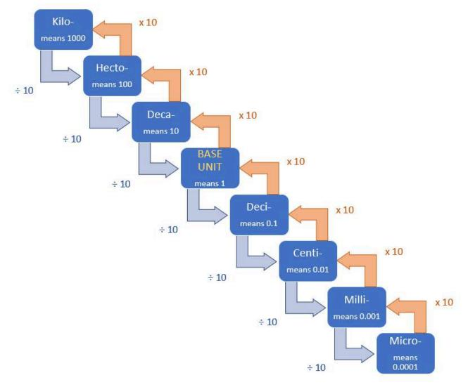
Figure 1. Unit measurement conversion flow chart.
