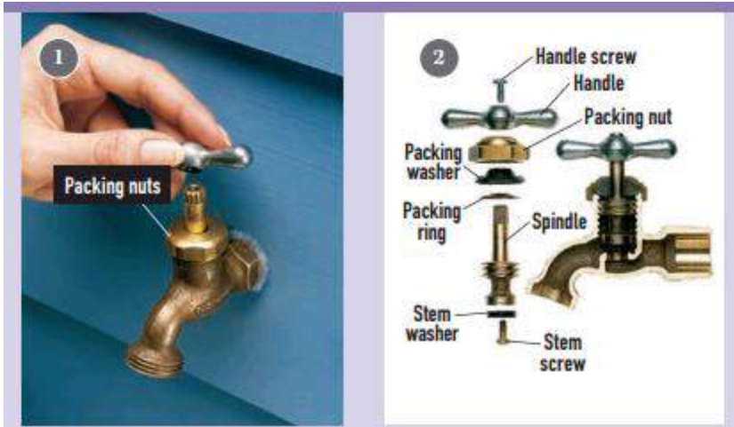
Figure 2.54 Components of hose bib
