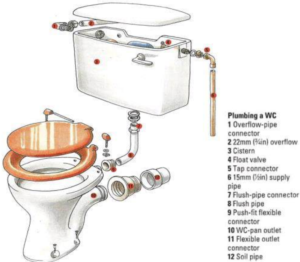
Figure 3.50 Detailed component of floor mount WC
