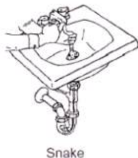
Figure 3.34 Clear up lavatory using snake
