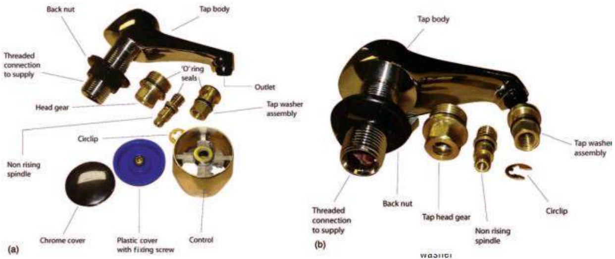
Figure 2.52 (a) Pillar tap components (b) Pillar tap seating and washer
