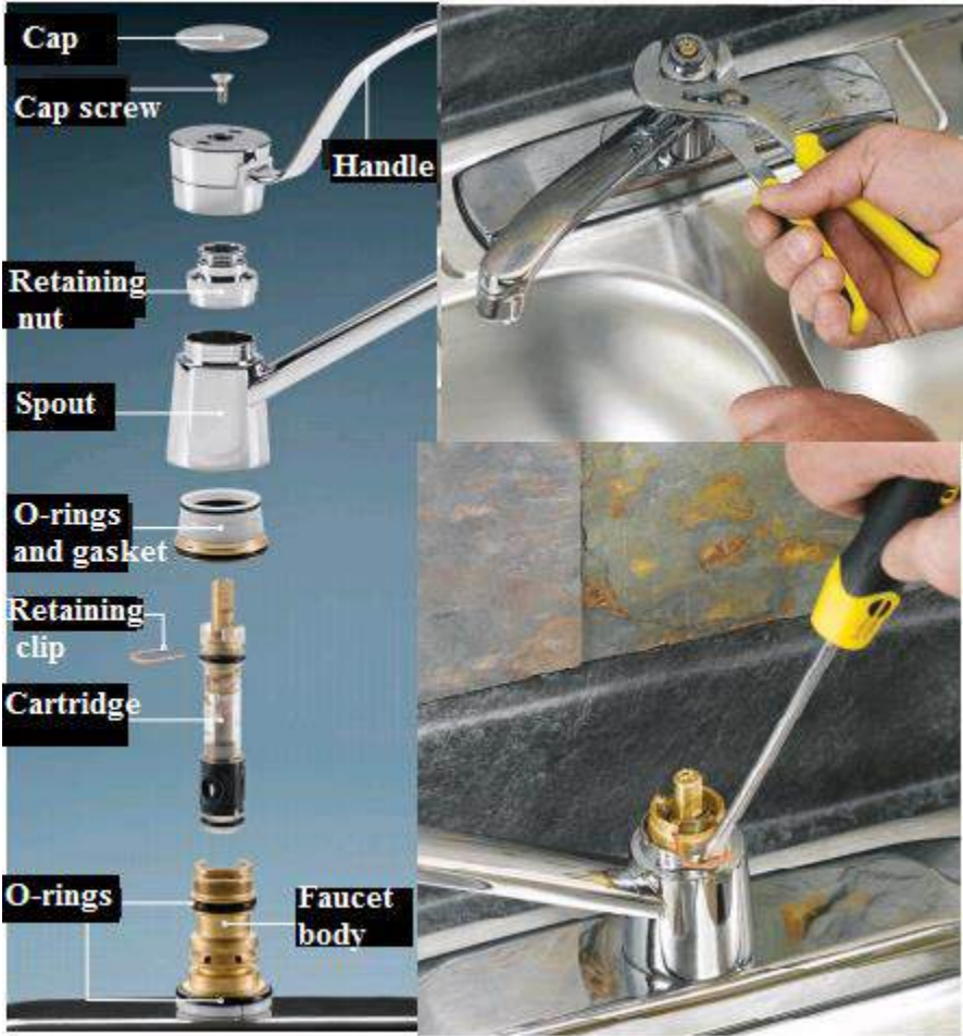
Figure 3.89 One-Handle Cartridge Faucets
