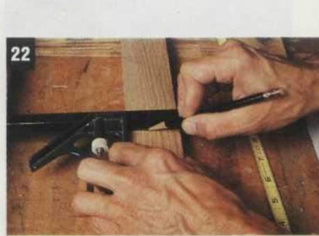
22 Measure an 11½" length on the 1" x 2" x 48" skirt piece. Square the mark and cut. Repeat for the remaining three skirt pieces. Now's the time to check the skirts and legs for blade burn, and sand the faces if needed.
