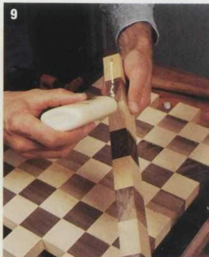
9 Using the same procedure as before, glue the eight strips together, in order, best face down, but shift every other strip by one block width to create the checkered pattern. Line up the cured joints carefully, because you won't get a second chance!
