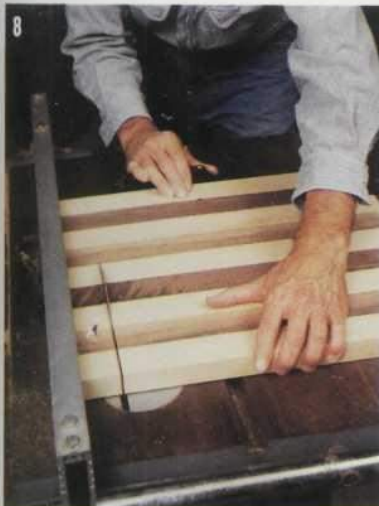
8 Reset the fence for a 1/4" cut and pass the board through the blade until you've got eight dark-and-light strips. Arrange them in the same order they've been cut.
