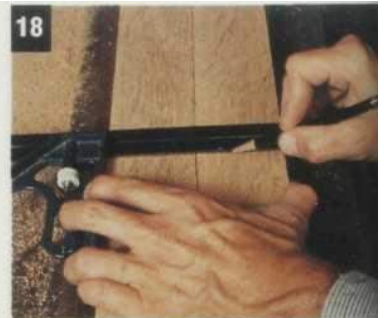
18 Use a square to carry the mark to the adjacent piece, then cut both. Repeat the procedure on remaining pieces to make four 19" leg blanks.
