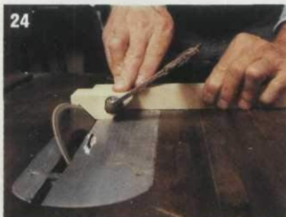
24 Tilt the table saw blade to a 45° angle and cut the four 1" x 1¼" x 2½" corner braces. Because the work is so close to the blade, clamp each brace to a scrap of 1 x 2 and make the cuts that way. Be sure the clamp clears the blade before starting the saw.
