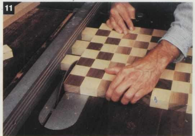
11 Use the saw's miter gauge to carefully trim the board to a 14" square.
