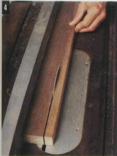
4 Rip the walnut into 1/4" strips and cut them into four 18" lengths.
