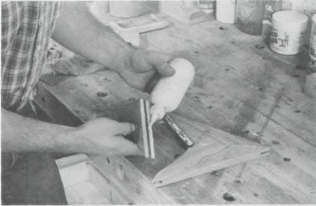
Glue and clamp triangles together.
