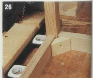
26 Glue the skirts to the legs, and the braces to skirts. If the corner braces don't set squarely against the skirts, place and draw up the cabinet screws lightly to hold the braces in place. Tighten the band clamp.
