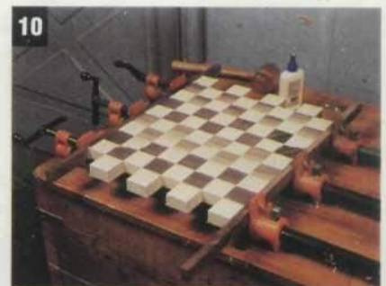
10 Clamp the board and allow the glue joints to cure for another 24 hours. Note the protective stickers at the clamps' heads and tails.
