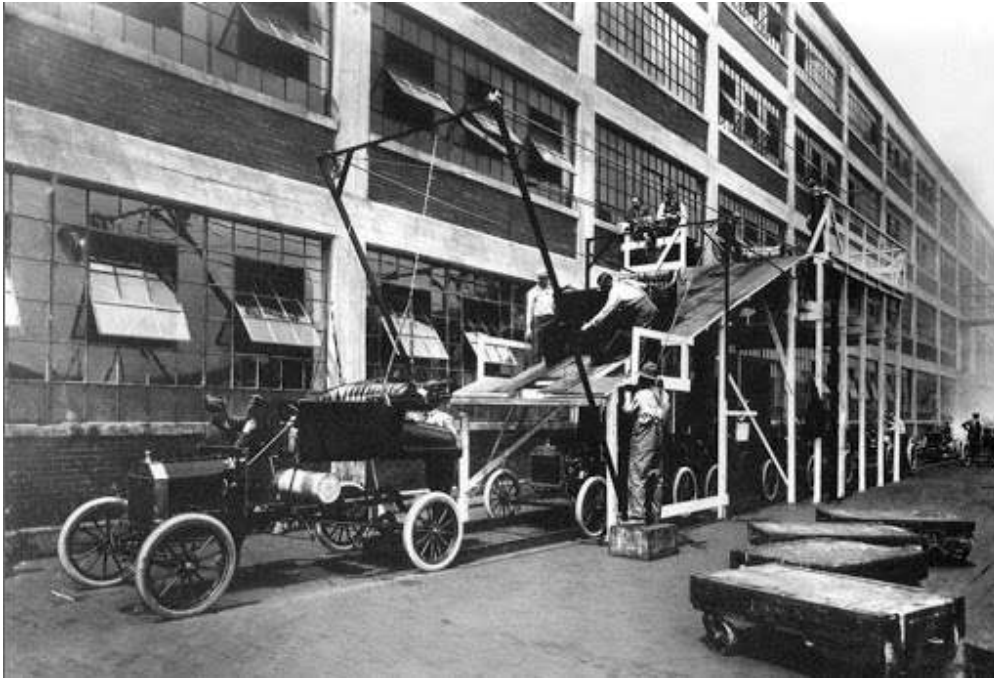
Figure 10.4: Division of labor was central to Henry Ford's development of assembly lines in his automobile factory. Ford noted, "Nothing is particularly hard if you divide it into small jobs."
