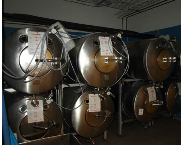
FIGURE 4.18 Fermentation of grape juice to make wine produces \text{CO}_2 as a byproduct. Fermentation tanks have valves so that pressure inside the tanks can be released.
