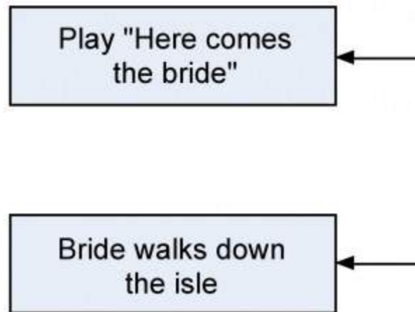
Figure 10.5: An example of a finish-to-finish (FF) predecessor.
