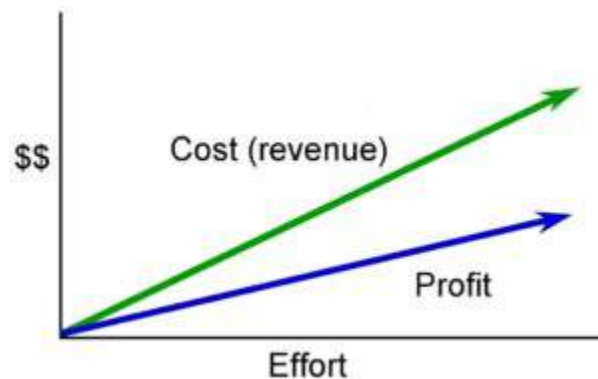
Figure 13.3: In a time-and-materials contract, the profit to the contractor increases with increased effort, as does the costs to the client.
