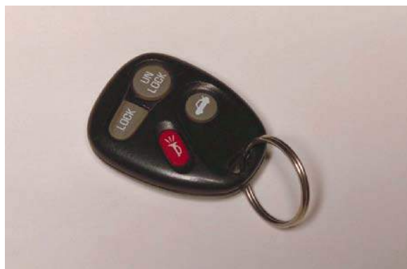
FIGURE 1-15 Remote keyless entry system transponder.
