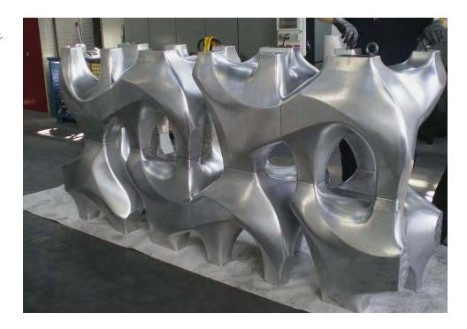
and by leveling. The surface was smoothed in several stages. The aluminum was then vacuum metallized in the vacuum chambers and passivated using the Chrome-Optics® procedure.
