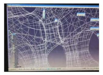
**Figure 2** Screen view of the digital mesh used to mill the shape of a preformed block in Anselm Reyle's aluminum sculpture *Philosophy*, 2009. Used with permission of Anselm Reyle. Photo: Thomas Dempwolf.
