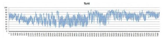
Figure 7d Relative humidity as recorded throughout the year of 2012 inside the same 1937 Mercury.
