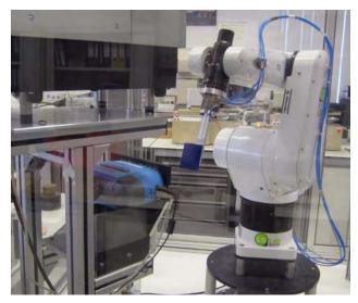
**Figure 4** An automated robot was used to take color and gloss measurements during and after aging tests at AkzoNobel. Photo by Nikki van Basten.
