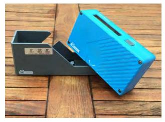
**Figure 9** A glossmeter is used to measure gloss of paint, plastic, paper, and other materials. The automobile industry is a primary user of glossmeters. Photo: J. Springvloet Dubbeld.
