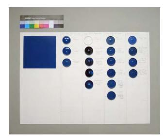
**Figure 3** Additives such as matting agents and colorants were added to the paint systems to alter color and gloss. Photo by Nikki van Basten.
