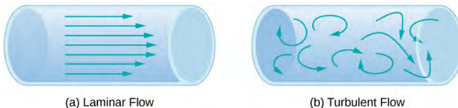
Figure 14.25 (a) Laminar flow can be thought of as layers of fluid moving in parallel, regular paths. (b) In turbulent flow, regions of fluid move in irregular, colliding paths, resulting in mixing and swirling.
