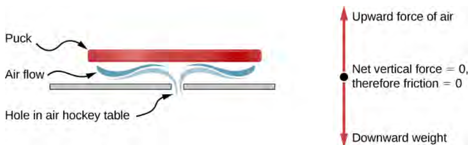
Figure 5.8 An air hockey table is useful in illustrating Newton's laws. When the air is off, friction quickly slows the puck; but when the air is on, it minimizes contact between the puck and the hockey table, and the puck glides far down the table.
