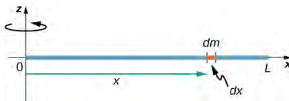
Figure 10.26 Calculation of the moment of inertia I for a uniform thin rod about an axis through the end of the rod.
