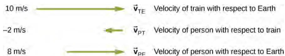
Figure 4.25 Velocity vectors of the train with respect to Earth, person with respect to the train, and person with respect to Earth.
