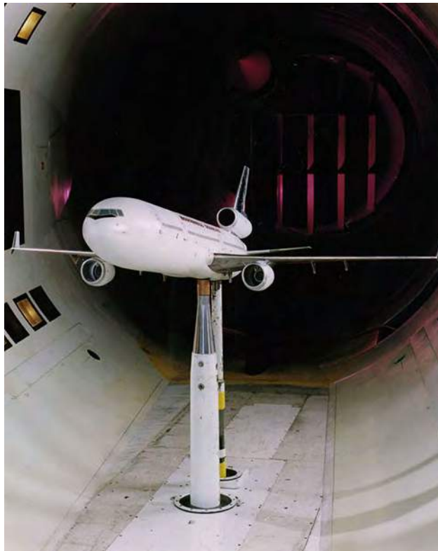
Figure 6.30 NASA researchers test a model plane in a wind tunnel. (credit: NASA/Ames)
