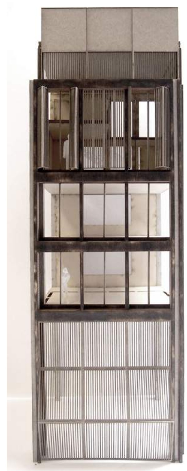
Fig 5.24 Laura Gaskell's study model of the aluminium curtain walling, shutters and structure of the London Makers Foundation, her award winning thesis project in Studio Mars at The University of Nottingham, 2013.
