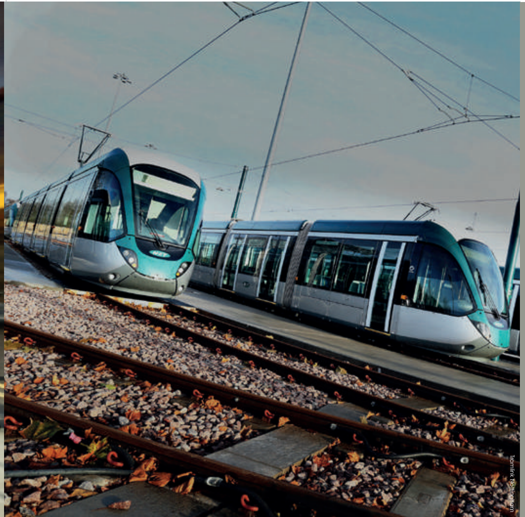
Reducing the weight of transportation vehicles is an important method of improving fuel efficiency – reducing energy consumption and greenhouse gas emissions. All aluminium bodied Alstom Citadis 302 Trams in Nottingham, England.
