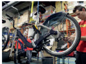
Aluminium is used by Cycles Devinci to manufacture the Bixi city sharing bicycles, designed by Michel Dallaire. They are used in bicycle sharing schemes including London, New York and Montréal.
