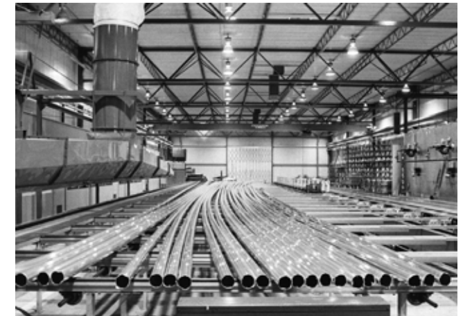
Fig 1.4 Extruded tubular sections, before straightening at Sapa, Tibshelf Plant, Derbyshire, England, architect, Foster Associates, 1973
