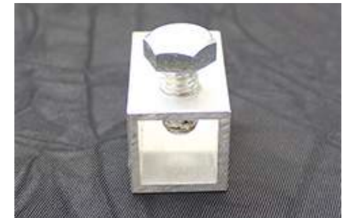
Fig 1.23 A Flowdrill port and aluminium bolt fixed through a small-extruded aluminium box section
