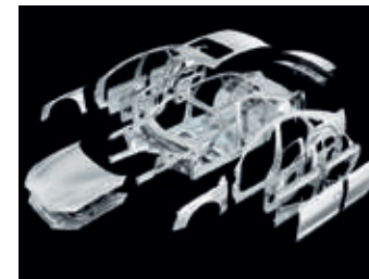
Lightweighting will increase intensity of use: in 2000 each automotive vehicle contained on average 100-120 kg of aluminium, in 2012 it was around 158 kg; by 2025 it is expected to be 250 kg.
