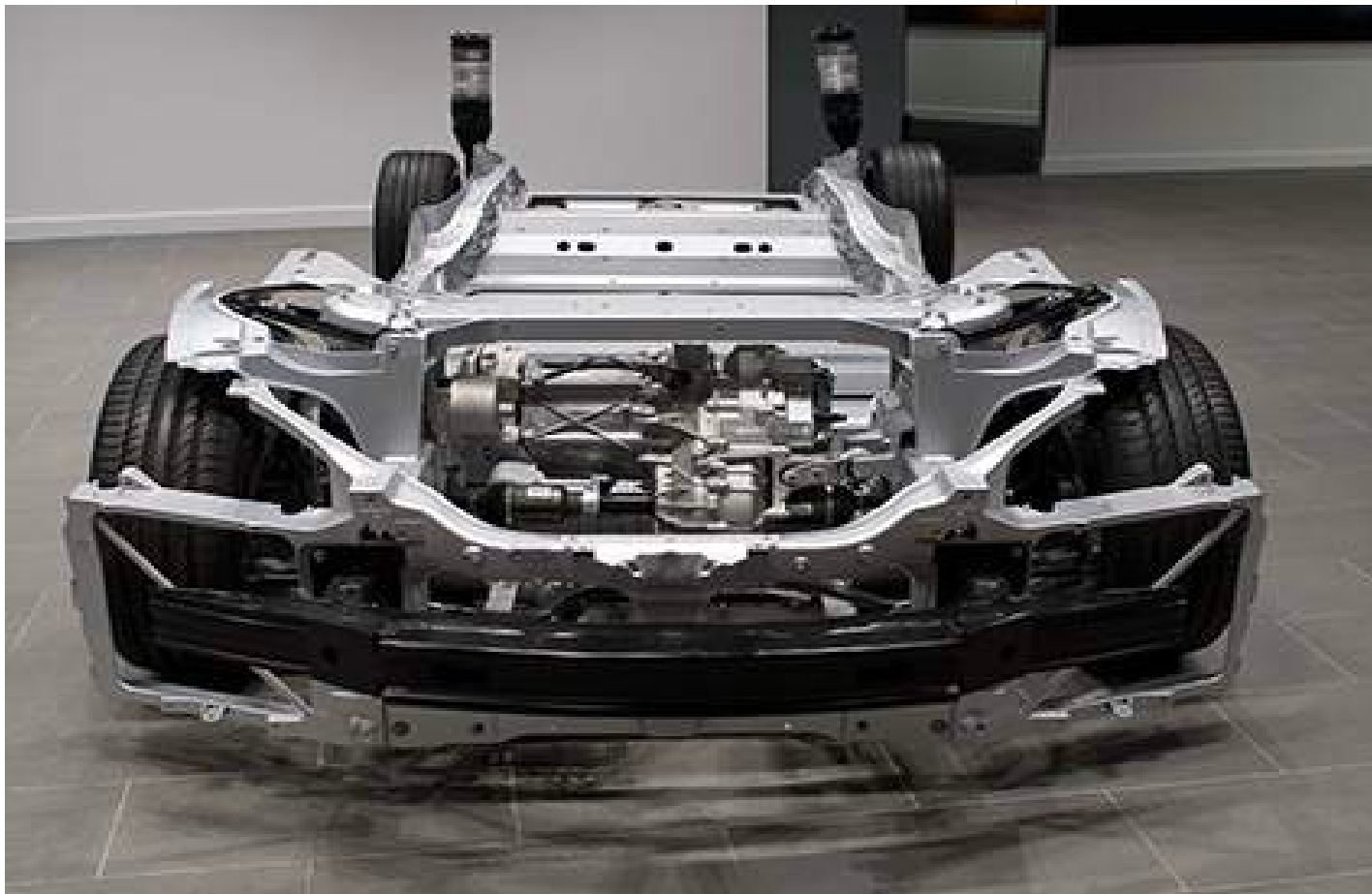
Fig 1.21 An aluminium alloy chassis, comprising sheet, extrusions and castings, which is common to both of Tesla's current electric cars, 2017
